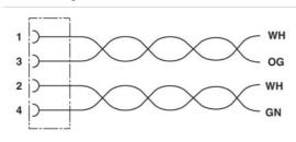
Contact assignment of the M12 socket
