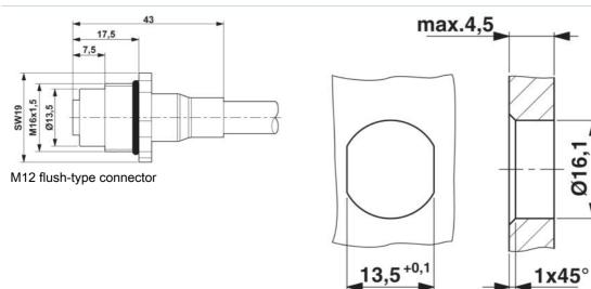
Housing cutout for M16 fastening thread, mounting panel with feed-through hole (alternatively with surface as protection against rotation) Circuit diagram
